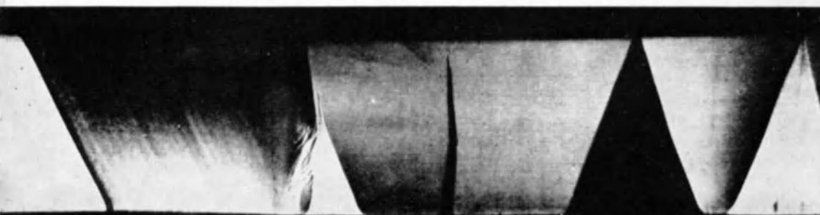
PLATE 5.2 (a) ( below ) Type A and (b) ( bottom ) Type B stretcher strains in annealed Al-3.5% Mg alloy strip. (Phillips et al. , 1952)
